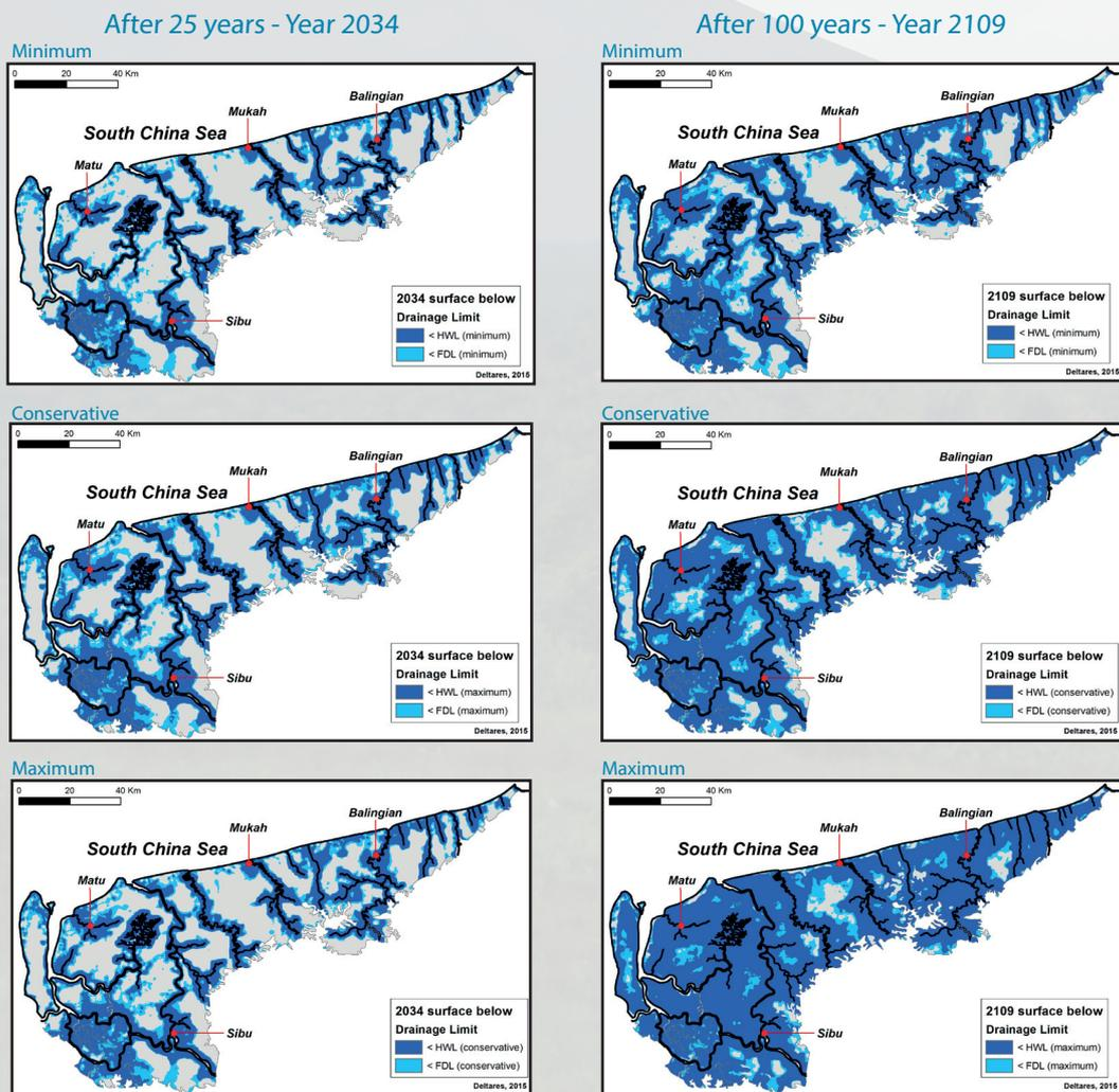
Figure 2: Comparison of flooding and drainability conditions according to the 'Minimum' (top), 'Conservative' (middle) and 'Maximum' (bottom) impact scenarios, after 25 (left) and 100 (right) years.
