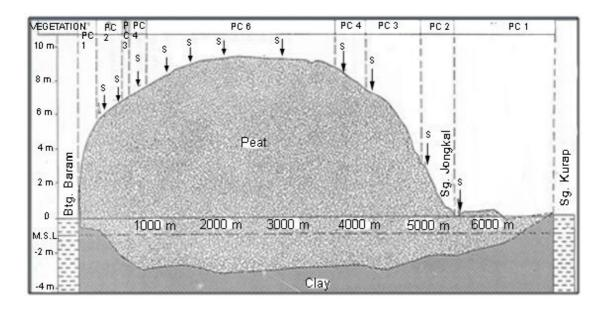
Figure 4: Cross-section of a peat dome close to Marudi showing how the base mineral soil is below mean sea level. Source: Tie (1990).
